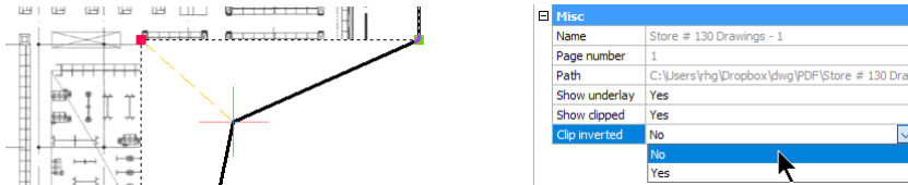
Left: Clipping boundary being edited with a grip; right: Inverting the clipping boundary
