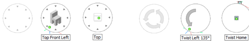
Left: LookFrom widget in isometric mode; right: ...and in Twist mode
